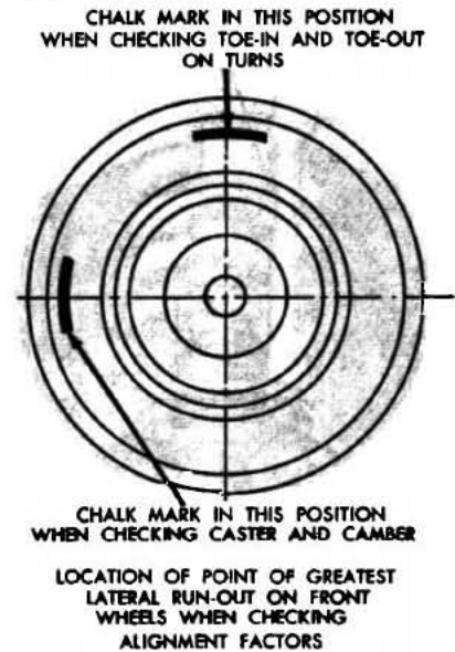
Fig. 74—Front Wheel Position for Checking Alignment
