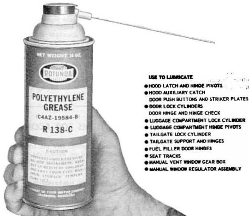
Fig. 105—Polyethylene Grease Dispenser for Body Lubrication
