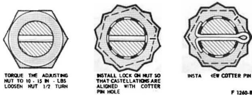
Fig. 94—Front Wheel Bearing Adjustment
